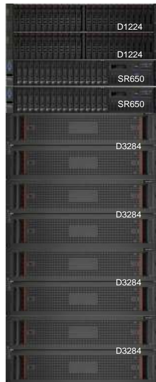
1 x DSS-G242 "hybrid" with both 2.5" SSD and 3.5" NL-SAS
